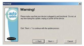
Note: It is crucial that the PC and the Switch remain powered-on, and the USB cable remains connected to the PC or the Switch during the update. The user should also avoid using the PC in ways that might interfere with the operations of the AutoUpdate application. If the update process is disturbed, the Switch could become nonfunctional. If the update is interrupted, but the Switch is still on, you should be able to restart the update (you may have to restart the AutoUpdate application).
